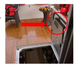
silver outer layer being the most noticeable. Marine inspectors subsequently wrote a deficiency after the vessel owner was unable to provide documentation proving the installed panels complied with 46 CFR 164.009. Insulation panels, particularly on vessels converted from recreational service, are often installed by the manufacturer or the owner for noise reduction purposes and may actually increase the risk of fire spread.
